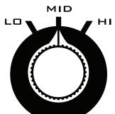
MID-HF LEVEL The selector switch is located on the back of each loudspeaker and provides the user the ability to tailor the output above 400Hz.
