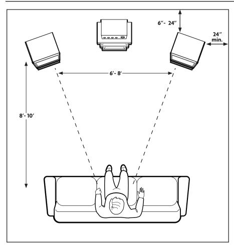
Room acoustics play a major role in the sound reproduction characteristics of your Model Five loudspeakers. Experimenting with loudspeaker placement is an important step for optimum acoustic performance and ensuring the customer gets exactly what they pay for. Fortunately, the Model Five is very placement friendly, and only a couple of factors need to be kept in mind:
