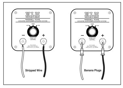
**IMPORTANT!** Turn your amplifier or receiver **OFF** before connecting your speakers. This will avoid damage which could result from accidental shorting of the speaker cables.
