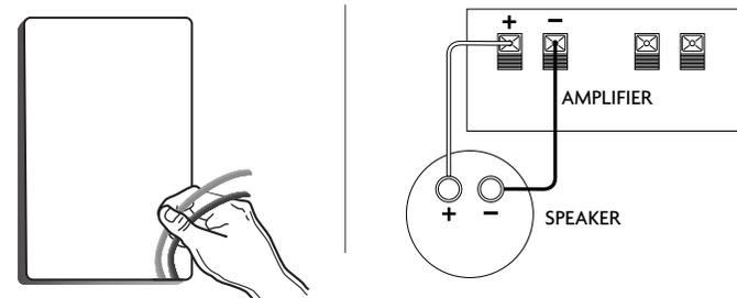
Place the speaker into the hole and press tightly against drywall with one hand, and tighten each of the screws until the speaker is firmly in place. Before placing grille on speaker, make sure there are no vibrations when playing. If so, check the installation screws to see if they need further tightening.
